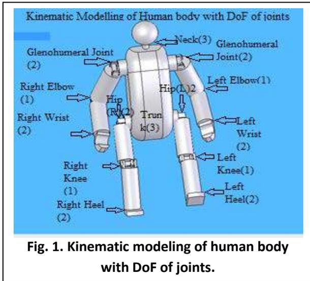
**Fig. 1. Kinematic modeling of human body with DoF of joints.**
