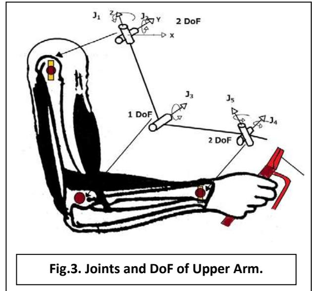
Fig.3. Joints and DoF of Upper Arm.
